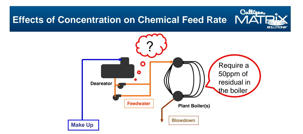
Boiler Residual / FW Cycles = Feed Rate
